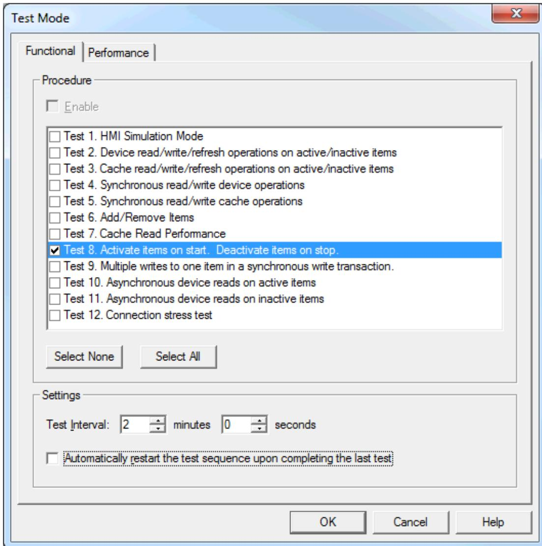
8. Return to **Tools | Test Mode** and disable test mode. All tags should be deactivated.
