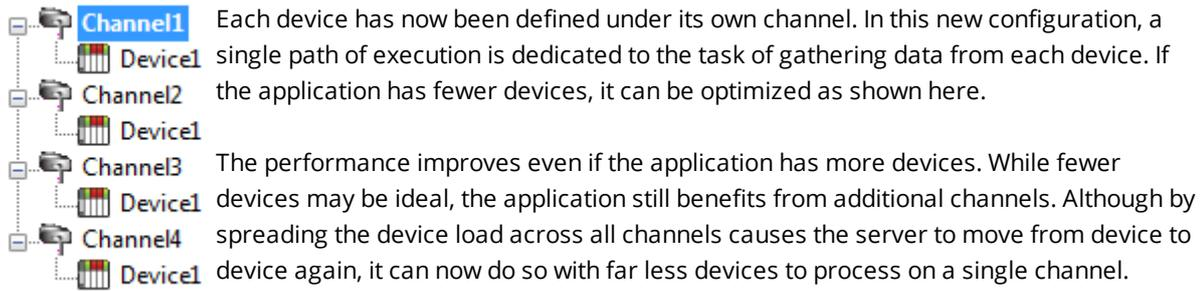
Each device has now been defined under its own channel. In this new configuration, a single path of execution is dedicated to the task of gathering data from each device. If the application has fewer devices, it can be optimized as shown here.
