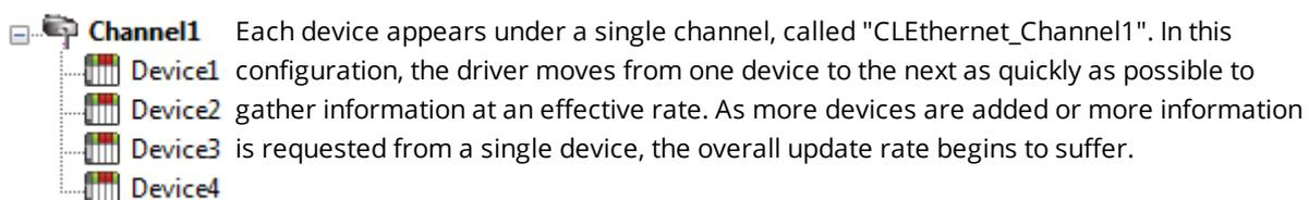
If the driver could only define a single channel, the example above would be the only option available; however, the driver can define up to 1024 channels. Using multiple channels distributes the data collection workload by simultaneously issuing multiple requests to the network. An example of how the same application may appear when configured using multiple channels to improve performance is shown below.
