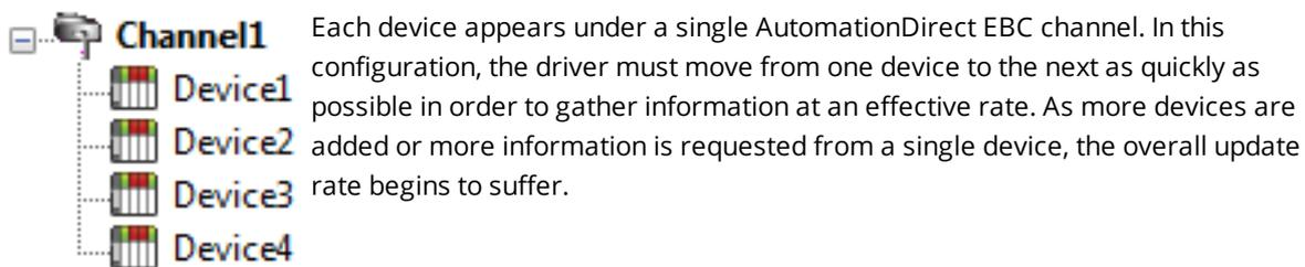
If the AutomationDirect EBC Driver could only define one single channel, then the example shown above would be the only option available; however, the AutomationDirect EBC Driver can define up to 100 channels. Using multiple channels distributes the data collection workload by simultaneously issuing multiple requests to the network. An example of how the same application may appear when configured using multiple channels to improve performance is shown below.
