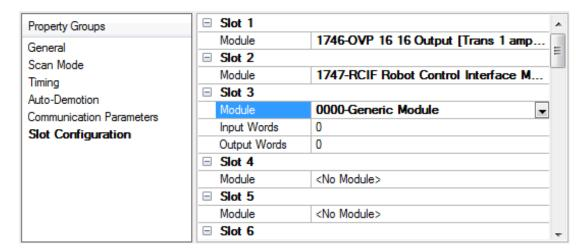
**Slot** *n*: the physical slot being configured. Use the plus icon to expand the properties.
