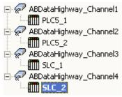
🖃 🐶 ABDataHighway\_Channel1 Each device has now been defined under its own channel. In this configuration, a single path of execution is dedicated to the task of gathering data from each device. If the application has 100 or fewer channels, it can be optimized as shown here.
