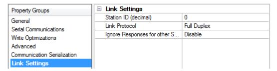
**Station ID**: The Station identity number is based on the device being communicated with (excluding radio modems):
