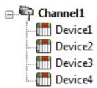
Each device appears under a single BUSWARE Ethernet channel. In this configuration, the driver must move from one device to the next as quickly as possible in order to gather information at an effective rate. As more devices are added or more information is requested from a single device, the overall update rate begins to suffer.
