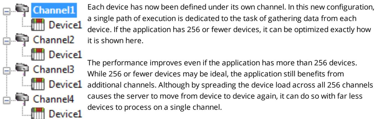
Each device has now been defined under its own channel. In this new configuration, a single path of execution is dedicated to the task of gathering data from each device. If the application has 256 or fewer devices, it can be optimized exactly how it is shown here.
