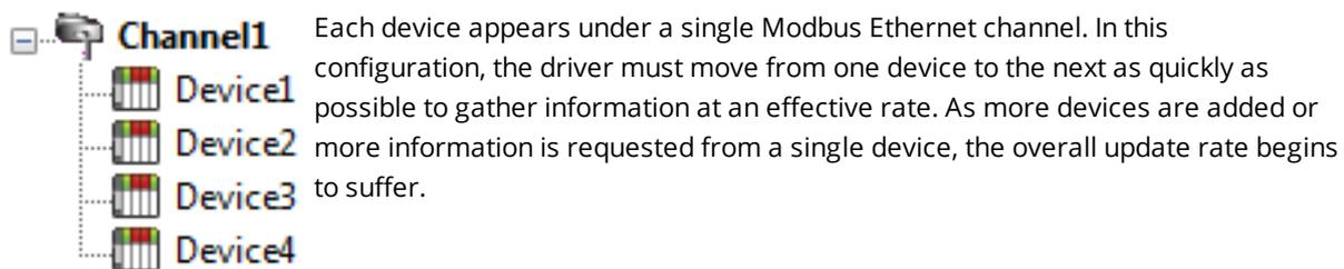
Each device appears under a single Modbus Ethernet channel. In this configuration, the driver must move from one device to the next as quickly as possible to gather information at an effective rate. As more devices are added or more information is requested from a single device, the overall update rate begins to suffer.
