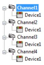
Channel1 Each device has now been defined under its own channel. In this new configuration, a single path of execution is dedicated to the task of gathering data from each device. If the application has 512 or fewer devices, it can be optimized exactly how it is shown here.
