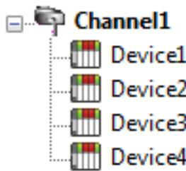
**Channel1** Each device appears under a single Wago Ethernet channel. In this configuration, the driver must move from one device to the next as quickly as possible in order to gather information at an effective rate. As more devices are added or more information is requested from a single device, the overall update rate begins to suffer.
