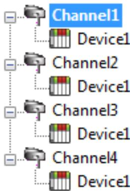
**Channel1** Each device has now been defined under its own channel. In this new configuration, a single path of execution is dedicated to the task of gathering data from each device. If the application has 16 or fewer devices, it can be optimized exactly how it is shown here.
