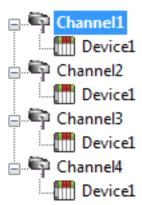
Each device has now been defined under its own channel. In this new configuration, a single path of execution is dedicated to the task of gathering data from each device.
