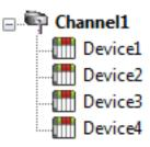
Channel1Each device appears under a single channel. In this configuration, the driver must<br/>move from one device to the next as quickly as possible in order to gather<br/>information at an effective rate. As more devices are added or more information is<br/>requested from a single device, the overall update rate begins to suffer.
