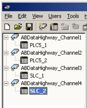
Each device has now been defined under its own channel. In this new configuration, a single path of execution is dedicated to the task of gathering data from each device. If the application has 100 or fewer channels, it can be optimized exactly how it is shown here.
