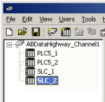
Each device appears under a single Allen-Bradley DH+ channel. In this configuration, the driver must move from one device to the next as quickly as possible in order to gather information at an effective rate. As more devices are added or more information is requested from a single device, the overall update rate begins to suffer.
