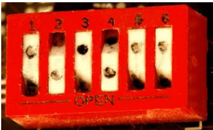
1. Configure the 1784-KT card DIP switches by pressing each switch in at the top or in at the bottom. Descriptions of the settings are as follows:
