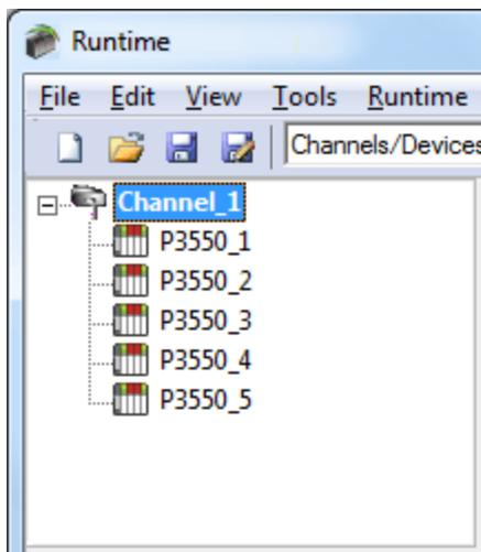
Each device appears under a single AutomationDirect Productivity Series Ethernet Driver channel. In this configuration, the driver must move from one device to the next as quickly as possible in order to gather information at an effective rate. As more devices are added or more information is requested from a single device, the overall update rate begins to suffer.
