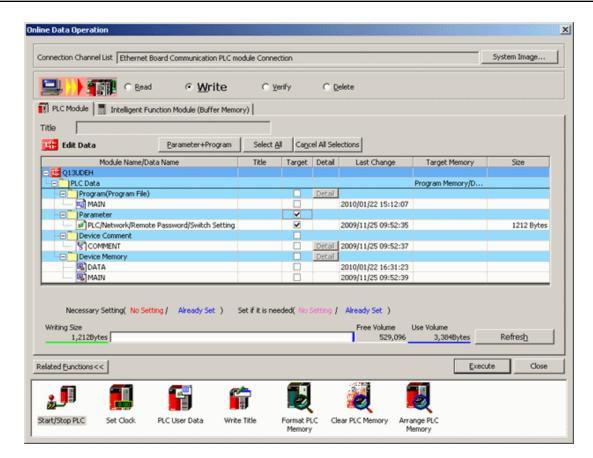
Note: Users must cycle the power on the PLC in order for the network parameter changes to take effect.
