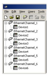
Each device has now been defined under its own channel. In this new configuration, a single path of execution is dedicated to the task of gathering data from each device. If the application has 256 or fewer devices, it can be optimized exactly how it is shown here.
