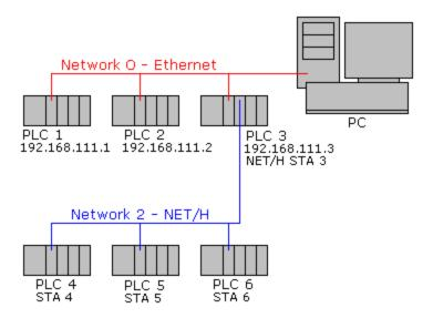
If PLC 1, PLC 2 and PLC 3 have QJ71E71-100 Ethernet modules configured with IPs 192.168.111.1, 192.168.111.2 and 192.168.111.3 respectively. In addition to the Ethernet module, PLC 3 also has a QJ71BR11 NET/H module configured as station 3. Assume that PLC 4, PLC 5 and PLC 6 have NET/H modules configured as stations 4, 5 and 6 respectively.
