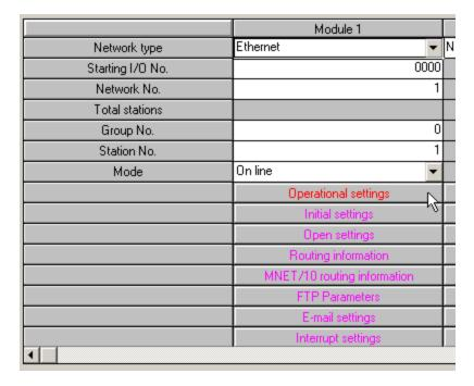
5. The **Ethernet Operations** dialog is used to define the device's IP address. Except for the IP address, the settings should be as shown below.
