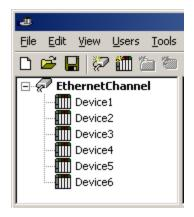
Each device appears under a single Mitsubishi Ethernet Device channel. In this configuration, the driver must move from one device to the next as quickly as possible in order to gather information at an effective rate. As more devices are added or more information is requested from a single device, the overall update rate begins to suffer.
