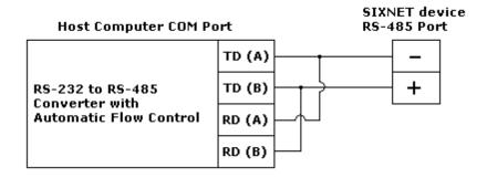
ST-CABLE-PF Cable for PC COM Port to RM-232-SETUP or RM-232-485-4U
