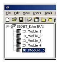
Each device appears under a single SIXNET UDR driver channel. In this configuration, the driver must move from one device to the next as quickly as possible in order to gather information at an effective rate. As more devices are added or more information is requested from a single device, the overall update rate begins to suffer.
