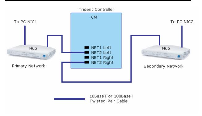
**Note:** Users can connect to NET1 or NET2. NET1 supports 10BaseT only. NET2 supports 10BaseT and 100BaseT.
