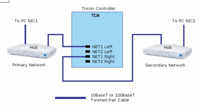
**Note:** For TCM models 4351A/4351B and 4352A/4352B, connect to NET1 or NET2. For TCM models 4353 and 4354, connect to NET1.
