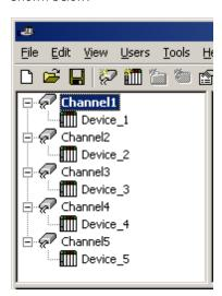
Each device has now been defined under its own channel. In this new configuration, a single path of execution is dedicated to the task of gathering data from each device. If the application has 32 or fewer devices, it can be optimized exactly how it is shown here.
