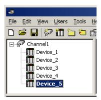
Each device appears under a single Triconex Ethernet channel. In this configuration, the driver must move from one device to the next as quickly as possible in order to gather information at an effective rate. As more devices are added or more information is requested from a single device, the overall update rate begins to suffer.
