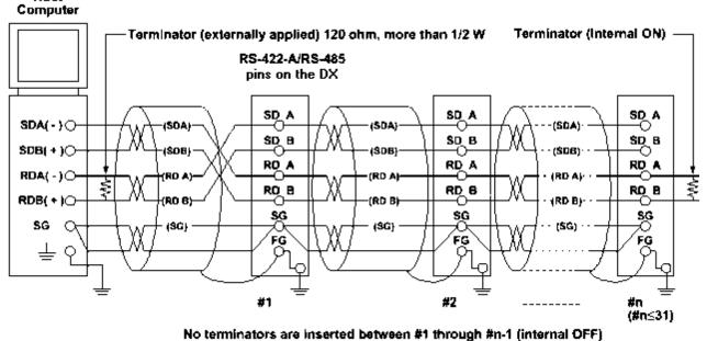
Note: RS-232 and RS-422 configuration is configured from the Yokogawa DX recorder's setup menu.
