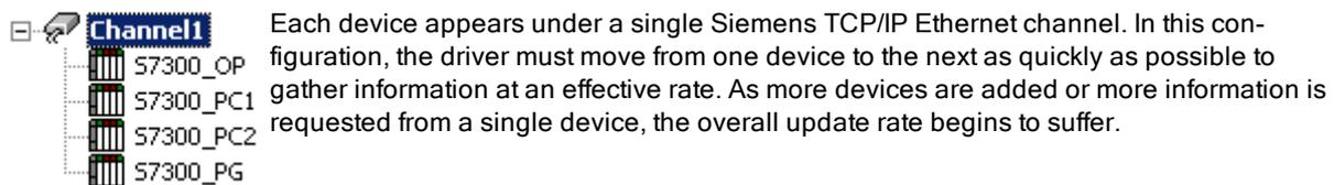
If the Siemens TCP/IP Ethernet Driver could only define one channel, then the example above would be the only option available; however, the driver can define up to 256 channels. Using multiple channels distributes the data collection workload by simultaneously issuing multiple requests to the network. An example of how the same application may appear when configured using multiple channels is shown below.
