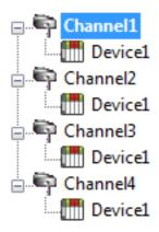
Each device has now been defined under its own channel. In this new configuration, a single path of execution is dedicated to the task of gathering data from each device. If the application has fewer devices than channels, it can be optimized exactly as it is shown here.
