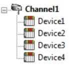
Each device appears under a single SIXNET EtherTRAK Driver channel. In this configuration, the driver must move from one device to the next as quickly as possible in order to gather information at an effective rate. As more devices are added or more information is requested from a single device, the overall update rate begins to suffer.
