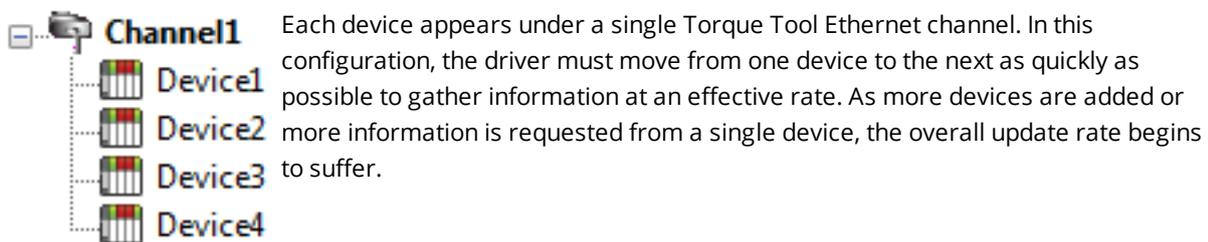
If the Torque Tool Ethernet Driver could only define one single channel, then the example shown above would be the only option available; however, the Torque Tool Ethernet Driver can define up to 100 channels. Using multiple channels distributes the data collection workload by simultaneously issuing multiple requests to the network. An example of how the same application may appear when configured using multiple channels to improve performance is shown below.
