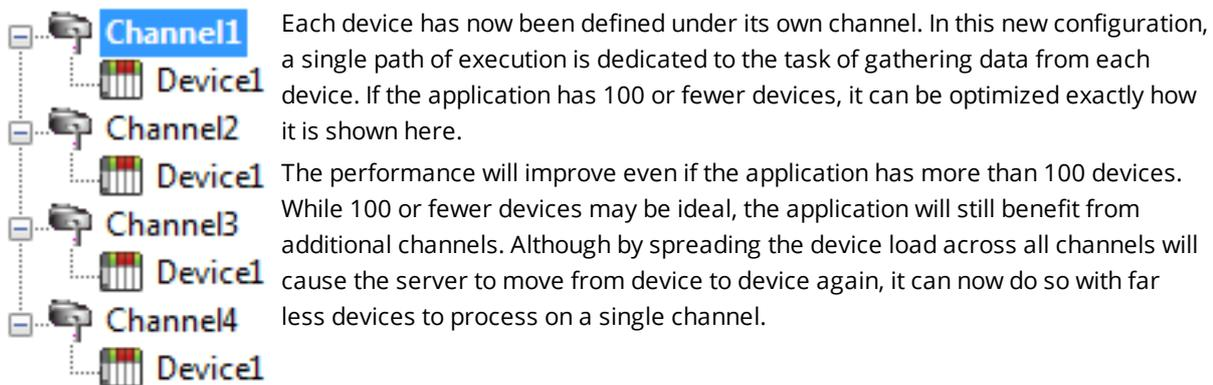
● **Note:** Some devices support only one Ethernet connection. For these devices, only one channel and device should be configured.
